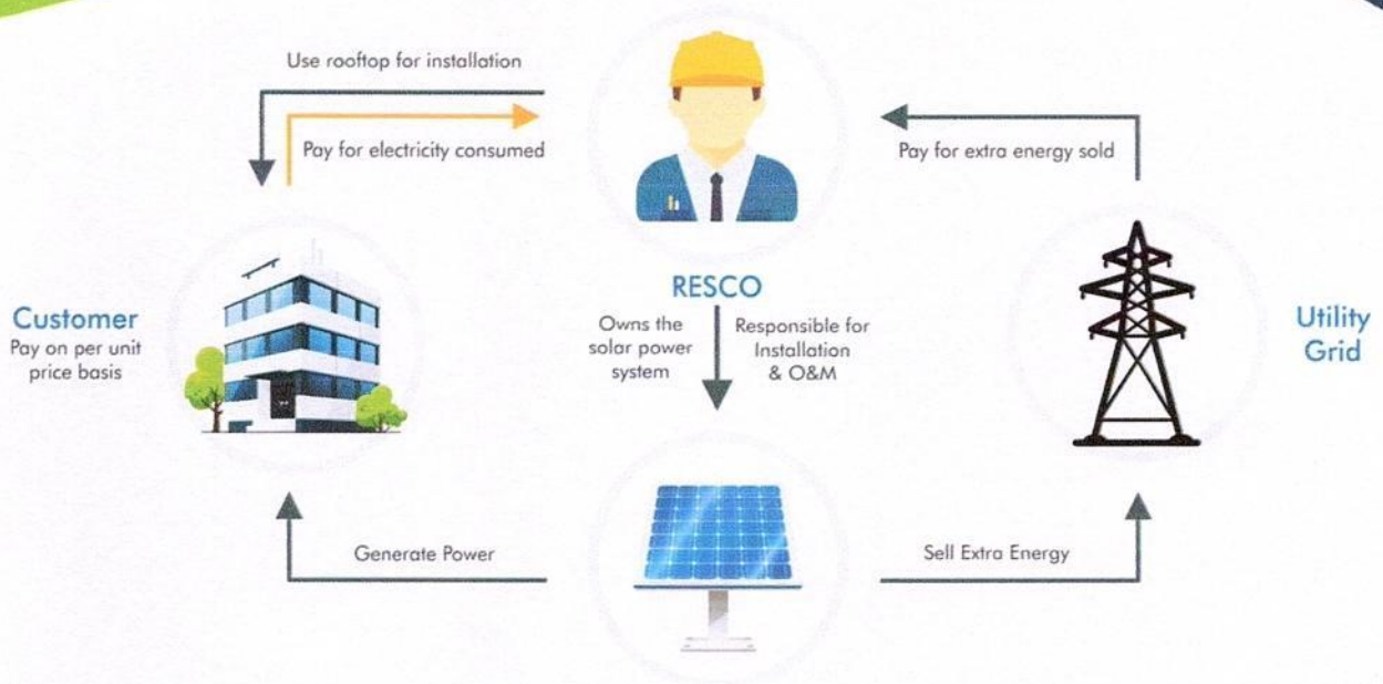
Solar Power Plant
